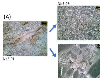
In the sedimentary rock sample, the rock images reveal distinct characteristics, including the presence of clay minerals (Fig 2. A) and variations in grain size. (Fig 2. B)
