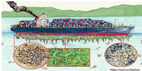
Fig. 2. In the absence of TBT usage, the hull tends to accumulate a multitude of organisms.
