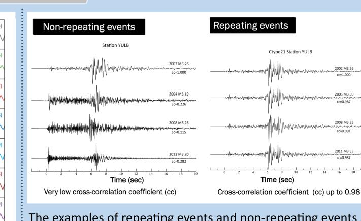
The examples of repeating events and non-repeating events at the same station. The former have nearly the same waveforms with high coefficient, while the latter have very low coefficient. Further more, the former are able to maintain their size and location over time, but the latter are not.
