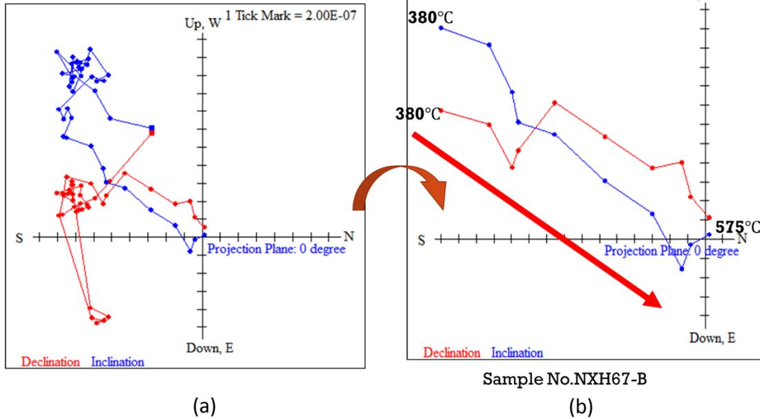
Figure 14. Zijderveld Diagram. (a) This diagram can show the direction of declination and inclination. (b) It shows one of recorded direction.
