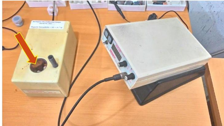
Figure 10. The instrument for the measurement of magnetic susceptibility. We put sample in the place where the arrow point at, then the sensor will show the value.
