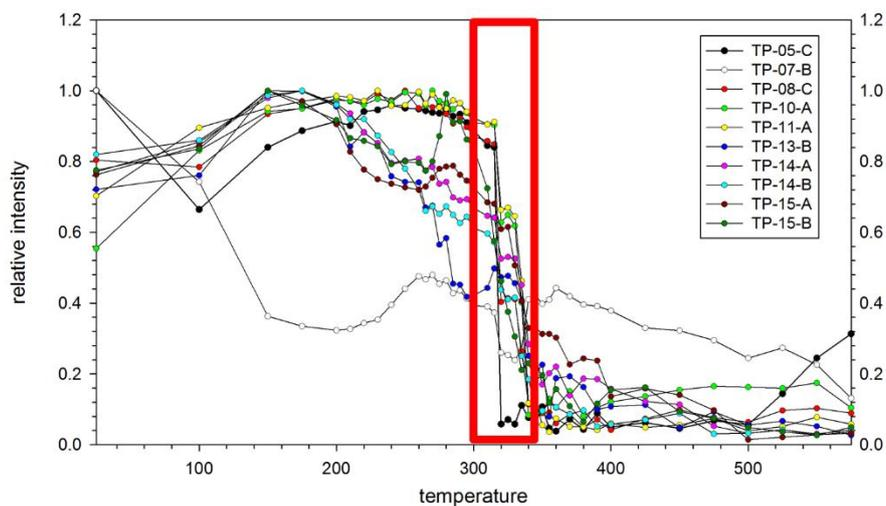
Figure 9. Relative Intensity with Temperature. The curve falls down quickly in a small interval of temperature. That means some remanent magnetization recorded by specific magnetic mineral has been removed.
