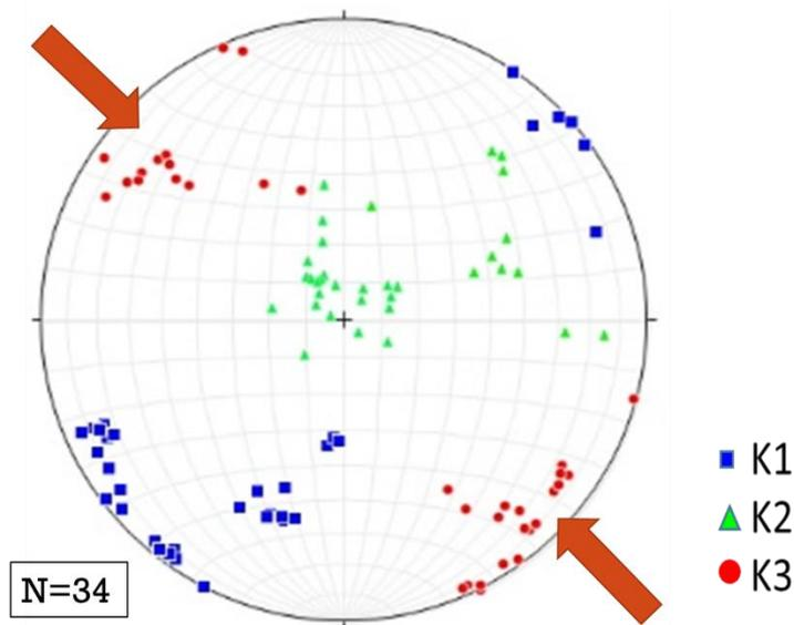
Figure 11. Stereonet plot. It indicates the NW-SE compression direction.
