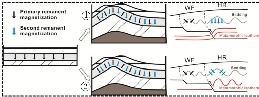
Figure 2. Fold Test. Case 1 is folding deformation before metamorphic temperature. Case 2 is folding deformation after metamorphic temperature. Fold test of remanent magnetization directions of rocks can separate these 2 cases.
