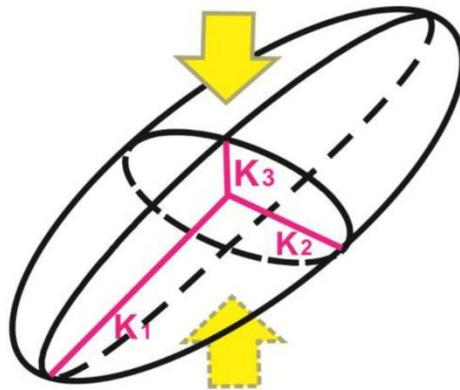
Figure 8. Magnetic susceptibility ellipsoid.  $K_1 \geq K_2 \geq K_3$
