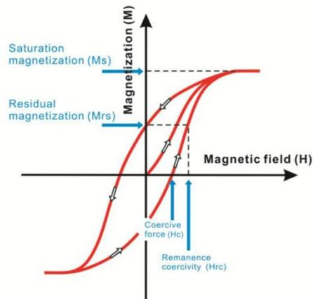
Figure 6. Hysteresis loop. Eye's shape in the middle means the existence of magnetic mineral.
