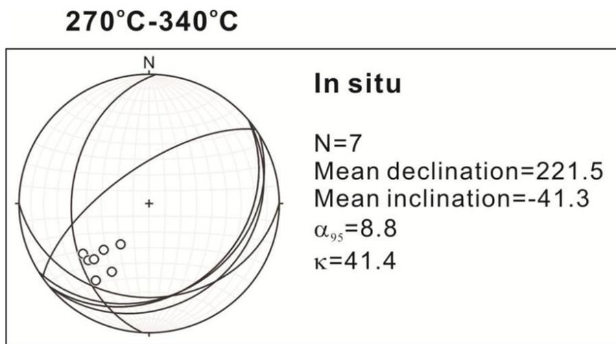
Figure 3. Stereonet Plot. Magnetic vectors are concentrated in the folding stage with reversal polarity.
