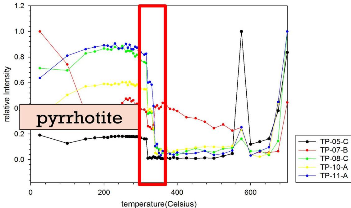
Figure 15. Intensity after normalizing. Relative intensity of most samples declined rapidly around 300-340 degrees , and exactly the Curie temperature of pyrrhotite is about 320 degrees.
