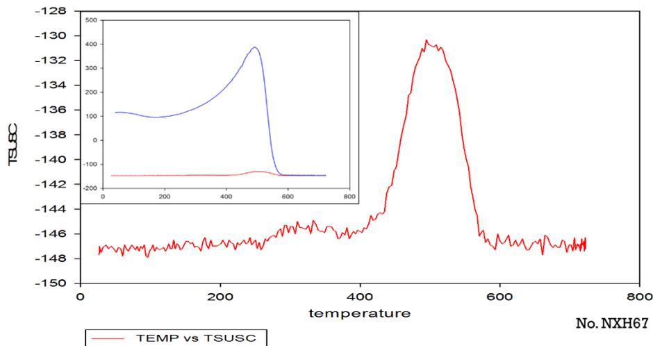
Figure 5. The plot of temperature with magnetic susceptibility. Red curve indicates heating, and blue curve denotes cooling.
